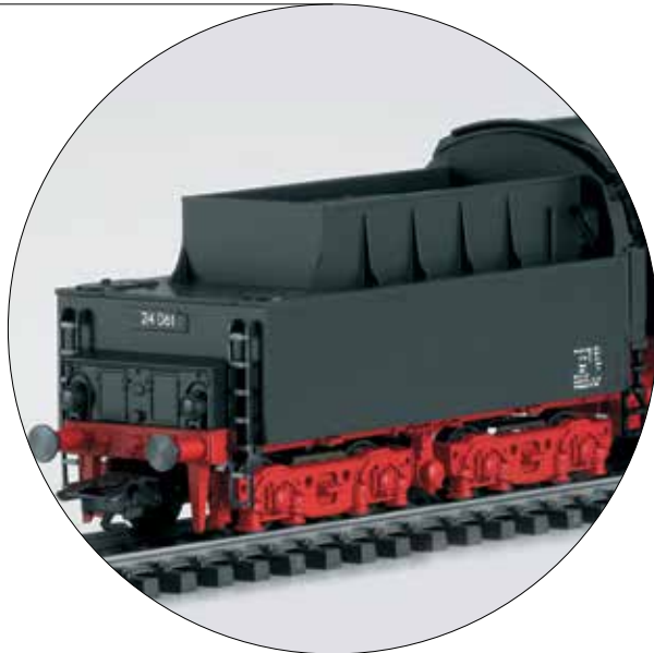
The 4-axle type 2'2'T26 was a guarantee in the prototype for smooth operation
