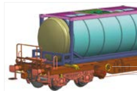
Separately mounted hand brake wheels and rods on the floor of the wagon / Volants de frein et timonerie rapportés
